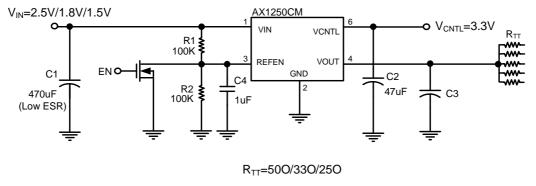
C3=10uF(Ceramic) + 1000uF under the worst case testing condition
