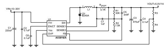
$$V_{OUT} = V_{FB} \times (1 + \frac{R1}{R2}), V_{FB} = 1.08V, R2 = 5K \sim 15K$$
