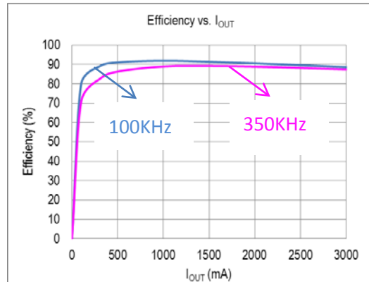
V CC =32V, V OUT =5V, I OUT =1A, C EN =0.1u, C OUT =22u x 2
