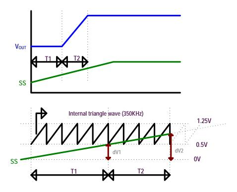
Start-up Delay Time: T1 =  $C_{SS} \times dV1/I_{SS}$ Soft Start Time: T2 =  $C_{SS} \times dV2/I_{SS}$
