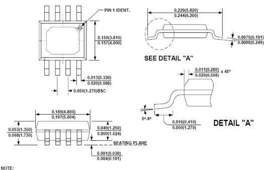
1) Control dimension is in inches. Dimension in bracket is millimeters.
