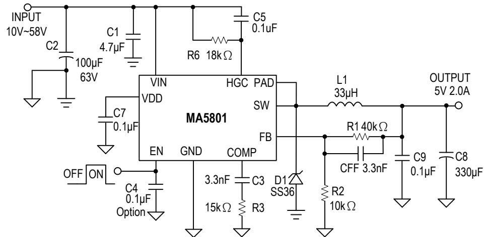
$$V_{OUT} = V_{FB} \times (1 + R1/R2), V_{FB} = 1.00V, R2 \text{ suggest } 1k\text{--}20k\Omega$$
