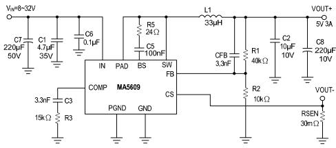
$V_{OUT}=V_{FB} \times (1+R1/R2)$ ,  $V_{FB}=1.00V$ , R2 suggest  $10k\sim40K\Omega$  $I_{SEN}=3.3A$  ( $I_{SEN}=VCS(0.1V)$  / RSEN( $30m\Omega$ ))
