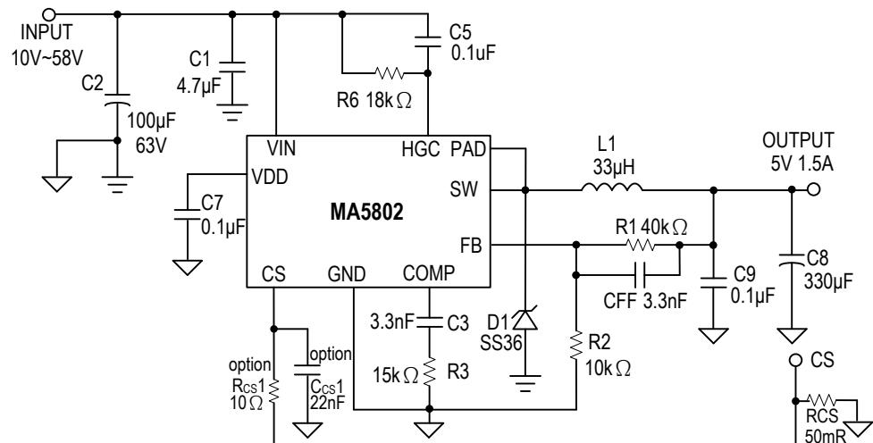
$$V_{OUT} = V_{FB} \times (1 + R1/R2), \quad V_{FB} = 1.0V, \quad R2 \text{ suggest } 1K \sim 20K\Omega.$$
