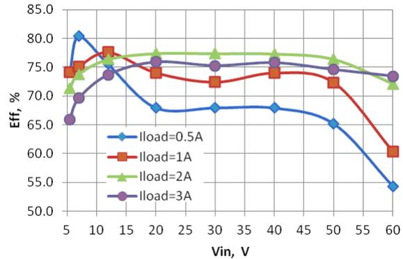
**Fig.5 Operating Efficiency**
