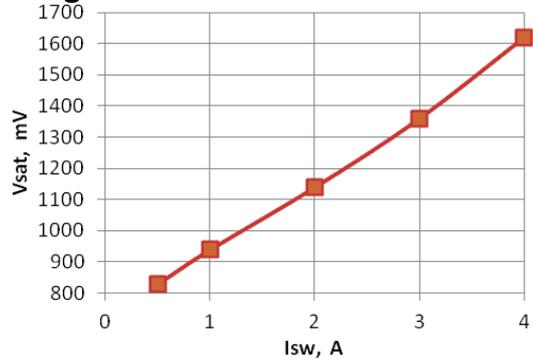
**Fig.3 Switch Saturation Voltage**
