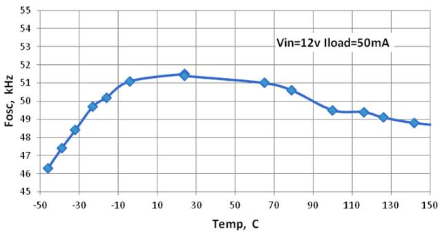
**Fig.4 Oscillator Frequency**
