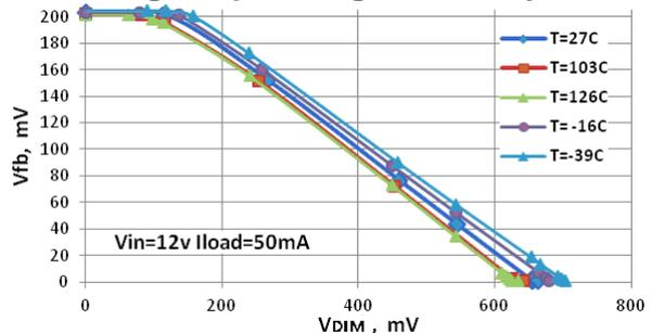
**Fig.7 Normalized Dimming Voltage**
