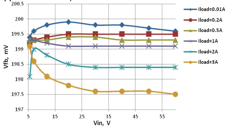
**Fig.1 Feedback Voltage**
